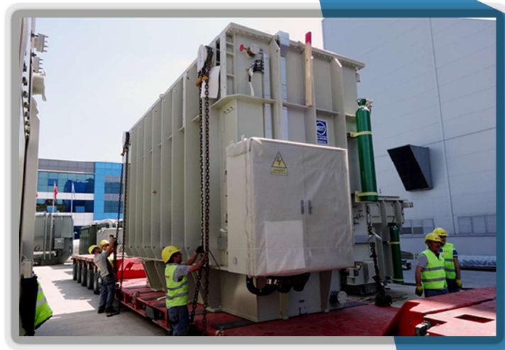
Pic. 3-4: SVC transformer before transport
