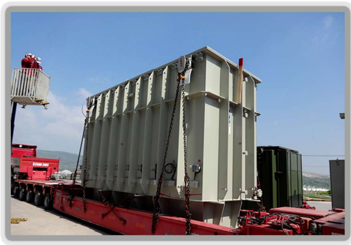
Pic. 3-4: SVC transformer before transport
