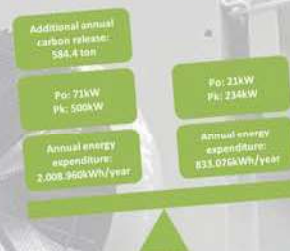
Pic 3 - Difference of yearly energy and carbon-dioxide emission between high loss and low loss 100MVA transformers (* under normal loading conditions)
