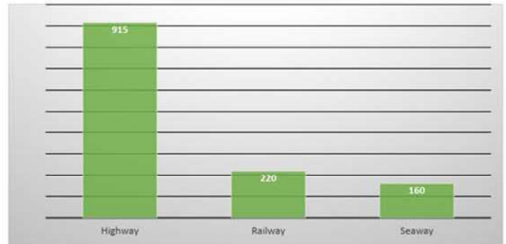
PIC 9 - Carbon emission values of a 200tonnes load which will be transported to 600km distance.[12]
