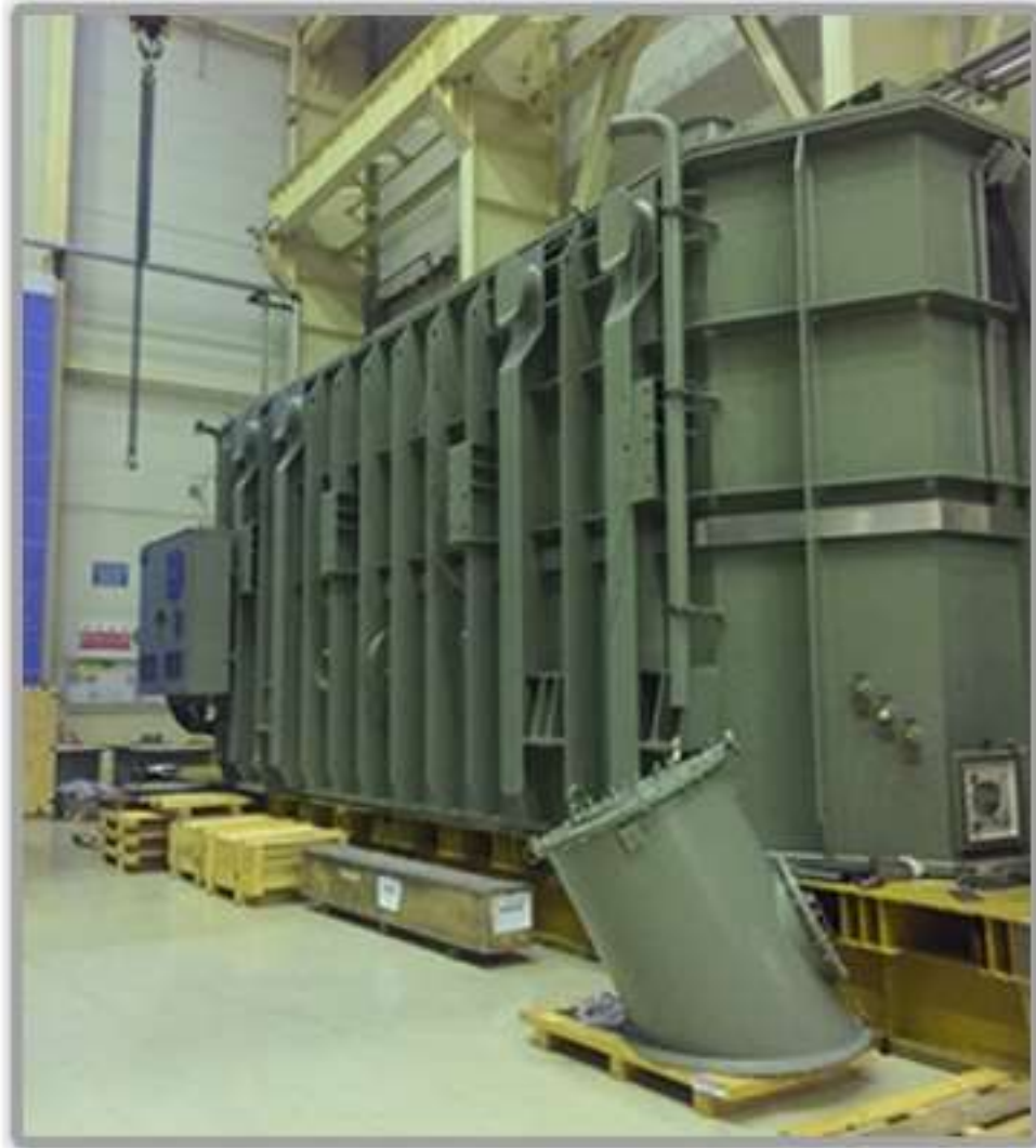
Pic. 4: All equipment removed before transportation.
