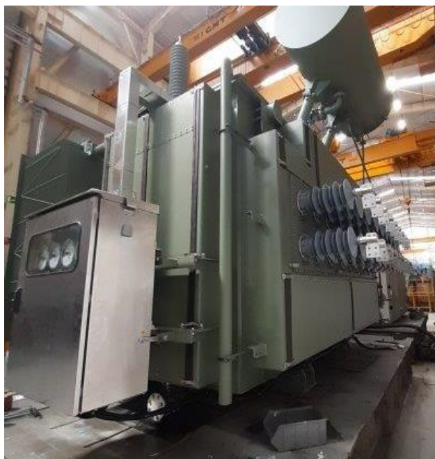
Figure 4 :Converter transformer before Factory Tests (FAT)
